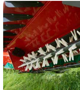
Efficient nylon tine conditioning.
