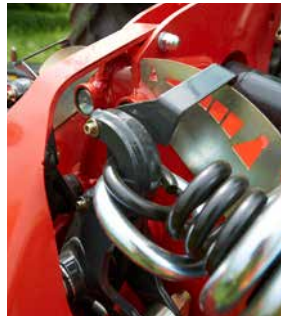
Large suspension springs, optionally with hydraulic setting of ground pressure.
