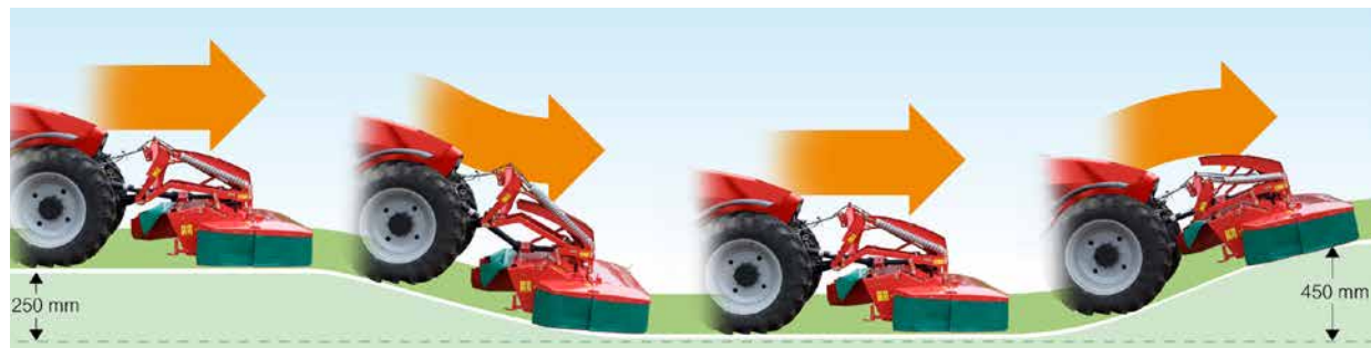
Excellent down- and upwards ground following ability of 250mm and 450mm respectively.
