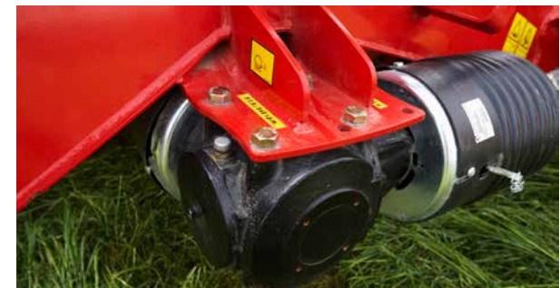
540/1000rpm turnable gearbox as standard.
