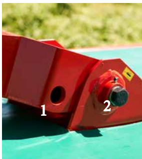
Two mounting positions of cutterbar on suspension for optimal overlap.
