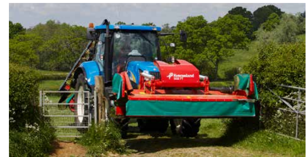
Foldable sideguards ensure narrow transport width.
