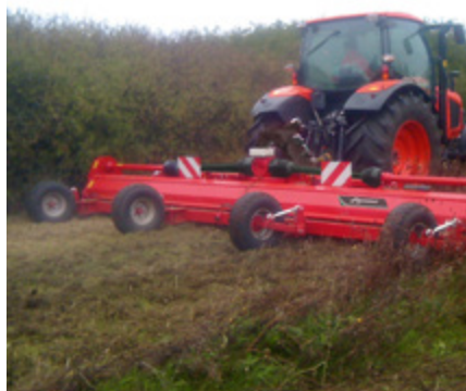
Semi pivoting wheels (10/8.0 x 12.8 ply) as option ensure a good stability and a constant working depth during field operations.
