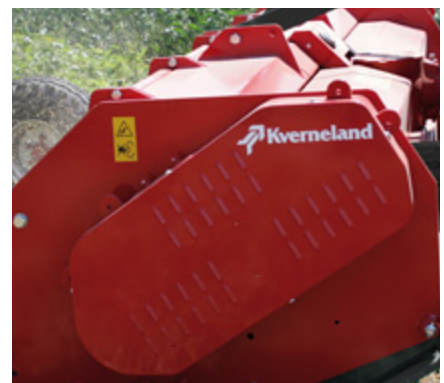
The FXZ is always equipped with a double lateral transmission. External and centralized greasing points of the rotor ensure a quicker maintenance.
