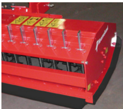
The Kverneland FHS can be equipped with rake tines to improve chopping on prunings.
