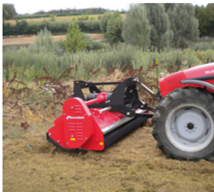
All gearboxes in Kverneland choppers range offer as standard integrated free wheel.
