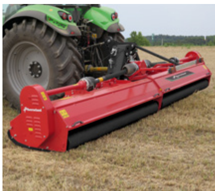
Working width from 560 to 640cm. The standard roller (Ø245mm) is running close to the profile to ensure a self-cleaning effect.
