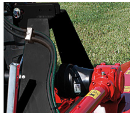
Gearbox up to 80hp - PTO speed drive 540 rpm. Protected by integrated free-wheel.
