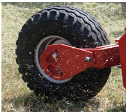
Semi pivoting wheels (10/8.0 x 12.8 ply) as standard ensure good stability and a constant working depth of the FXZ during field operations.
