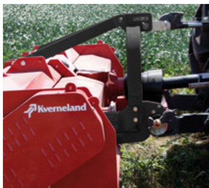
Semi automatic linkage (Cat III) allows fast coupling of FXZ. In addition the floating top link mounting permits easy control of the working depth without stressing force on the headstock.
