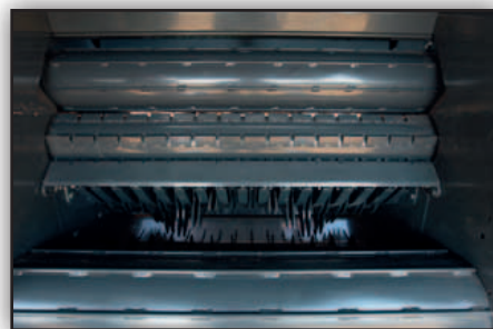
The bale chamber concept consists of 5 rollers at the front...
