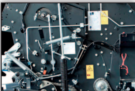
Steel pipes for hydraulic circuits.
