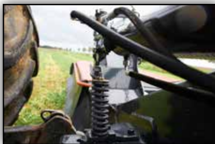
When encountering an obstacle the NonStop BreakAway system protects the cutterbar by swinging it back and up.
