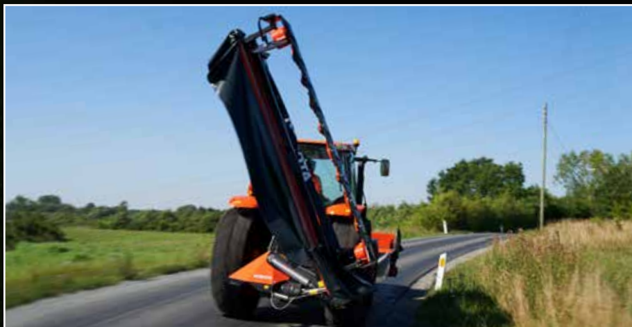
Up to 125° vertical transport position for excellent weight distribution.
