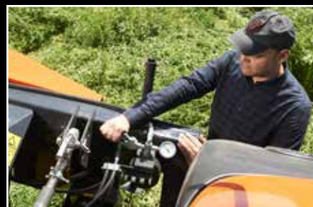
Hydraulic setting of ground pressure.
