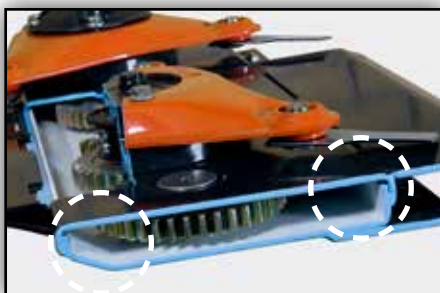
Fully welded cutterbar with overlapping C-channels for a very strong and stiff construction.
