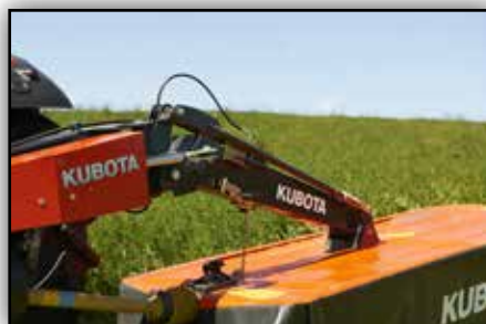
Centre mounted suspension for even weight distribution and fast adaptation to ground contours.
