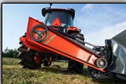
Four v-belts ensure excellent transfer of power.
