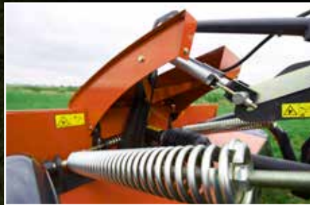
Two springs provide excellent ground following ability.
