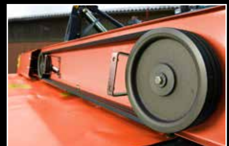
By switching driveline pulleys changing from standard PTO speed of 1000 rpm to 750 rpm is possible.
