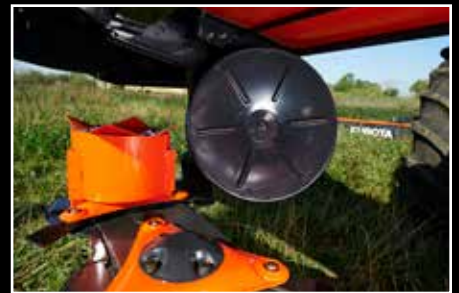
The machine is standard equipped with two swath discs, allowing a swath width of 2.2-2.4m.
