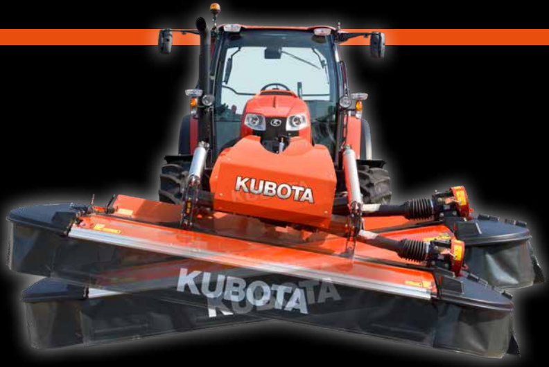
Vertical adaptation of 24° to adjust to uneven fields.
