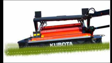
The suspension springs ensure excellent sideways adaptation of the complete mowing section.
