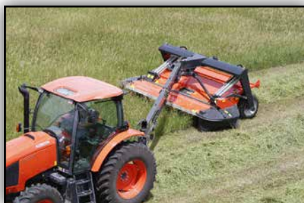
The mower can be operated on either side of the tractor....
