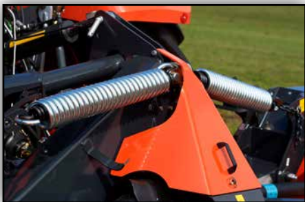
Large suspension springs, optionally with hydraulic setting of ground pressure.
