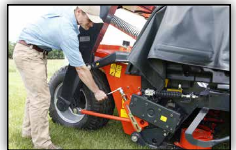
Easy adjustment of stubble height.
