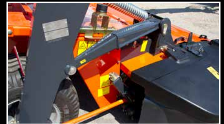
When an obstacle is encountered, the mowing section is forced backwards and the special suspension rod ensures that the mowing section is automatically lifted upwards and above the object.
