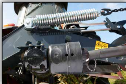
Two speed gearbox – switched by turning the main gearbox 180°.
