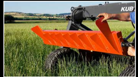
Changing from swathing to wide spreading is a one-man job. Simply turn the rear plate 180°.
