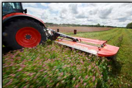
Centre suspension for even weight distribution across the entire working width.
