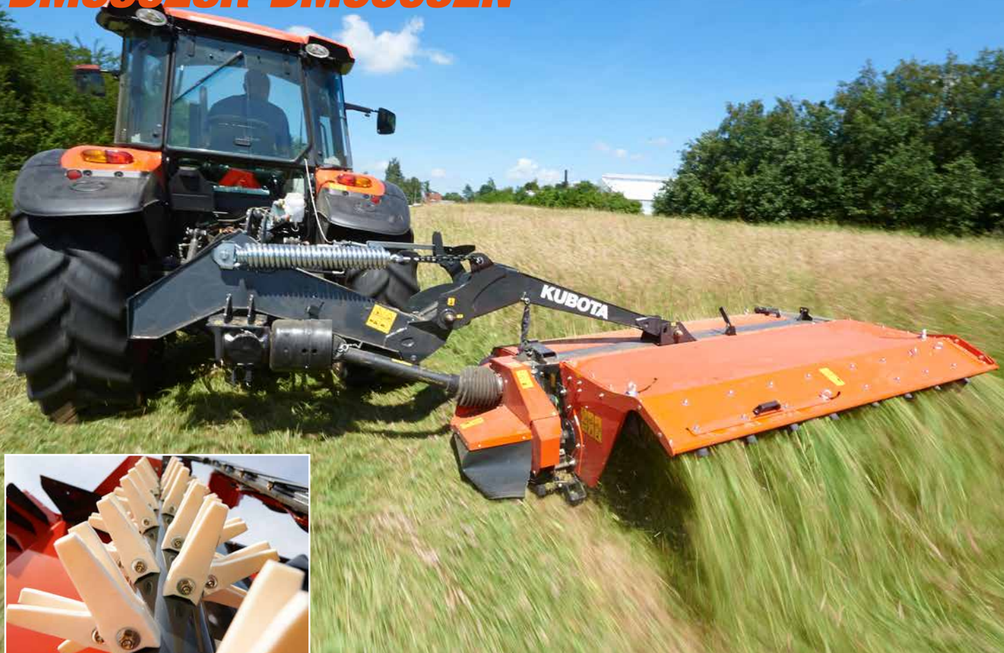
Effective 600/900 nylon tine conditioning.
