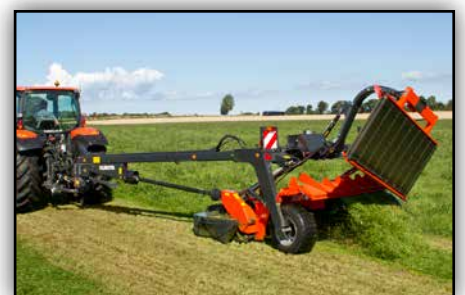
When placing the first swath, the belt is raised and hydraulically lowered for the second swath.
