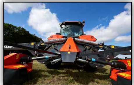
Large compensating spring ensures excellent flotation across the full mower width.
