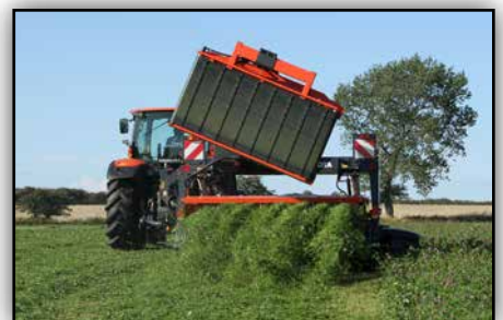
The crop is directed inwards, away from the unmown crop.
