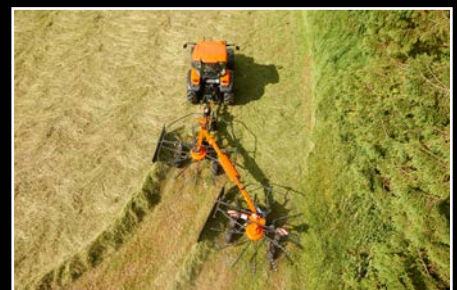
Both rakes are capable of placing small night swaths for hay crops.
