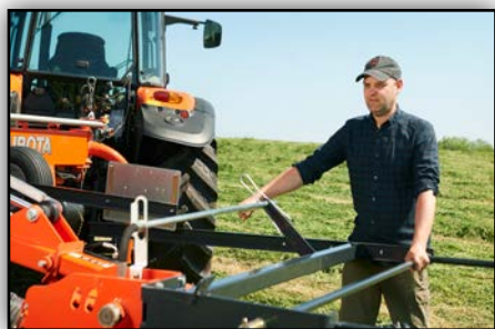
Easy setting of correct raking height.
