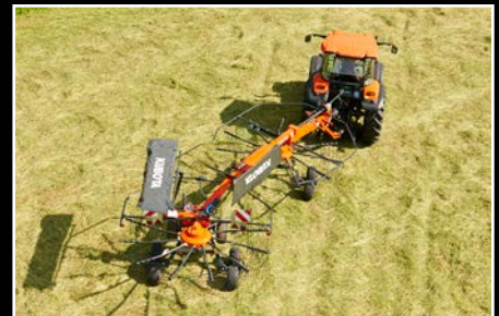
SideShift to the left - raking without driving on unraked crop.
