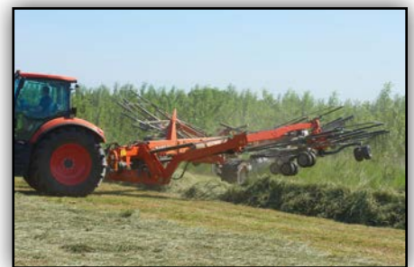
High lift of rotors ensures generous clearance during headlands turns. Clearance height can be adjusted infinitely.
