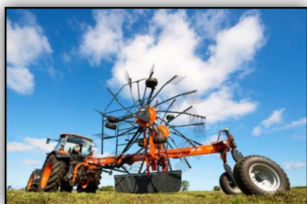
Kubota RA2584 is converted hydraulically for transport position from tractor cab.
