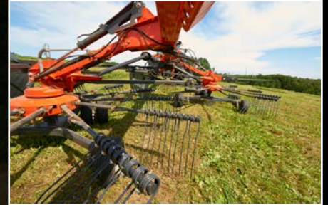
Generous overlap between rotors ensures clean raking.
