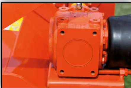
Gearbox with integrated free wheel.
