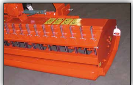
The Kubota SE3000 series can be equipped with rake tines to improve chopping on prunings.
