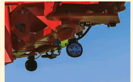
Boom lights (LED) For the best view of the boom and crop, when spraying at night.
