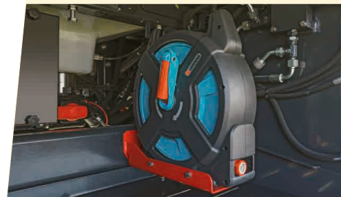
Sensing skid Prevents the spray boom from touching the ground.
