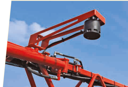
Boom Guide Automatic spray height control.
