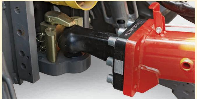
A pulling eye of  $\varnothing$  40/50mm for low or top linkage or ball coupling  $\varnothing$  80mm for safe and firm hitching available.
