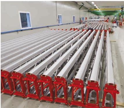
The high tech aluminium boom production location is a closed and ultra clean environment with climate control and pressurisation to guarantee ideal conditions and top quality for the gluing procedure of our famous aluminium booms. Focus is given in all production processes to trainings and certifications of people to ensure a high quality standard of Crop Care products.
