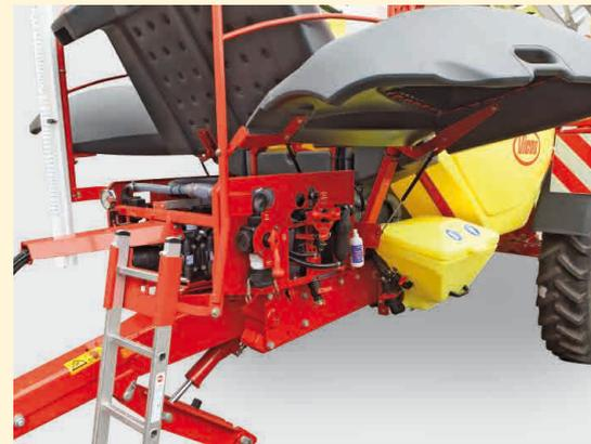
The covers are giving easy access to the control panel and operator functions. Special attention has been put on service friendliness by easy access and quick-fit hose connections.
