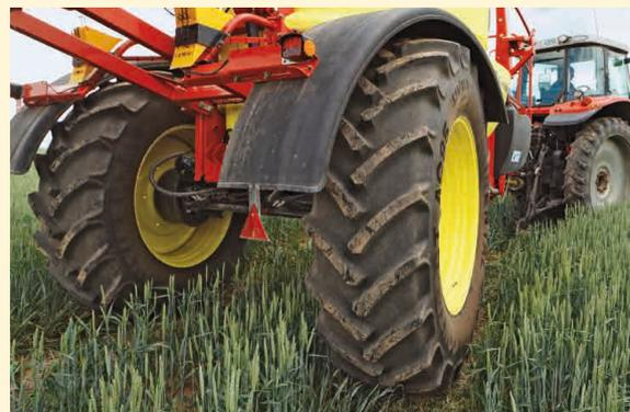
Suspended steering axle (iXtrack C30/C40/C50)
