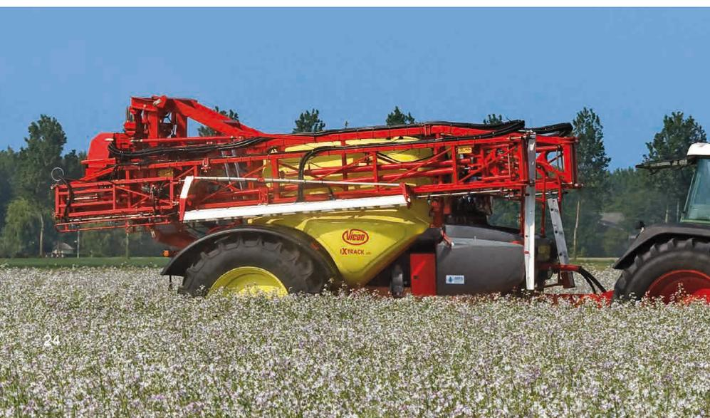
The strong parallelogram system with two lifting cylinders gives an optimum spraying height and no torsion whilst folding the boom in and out.
