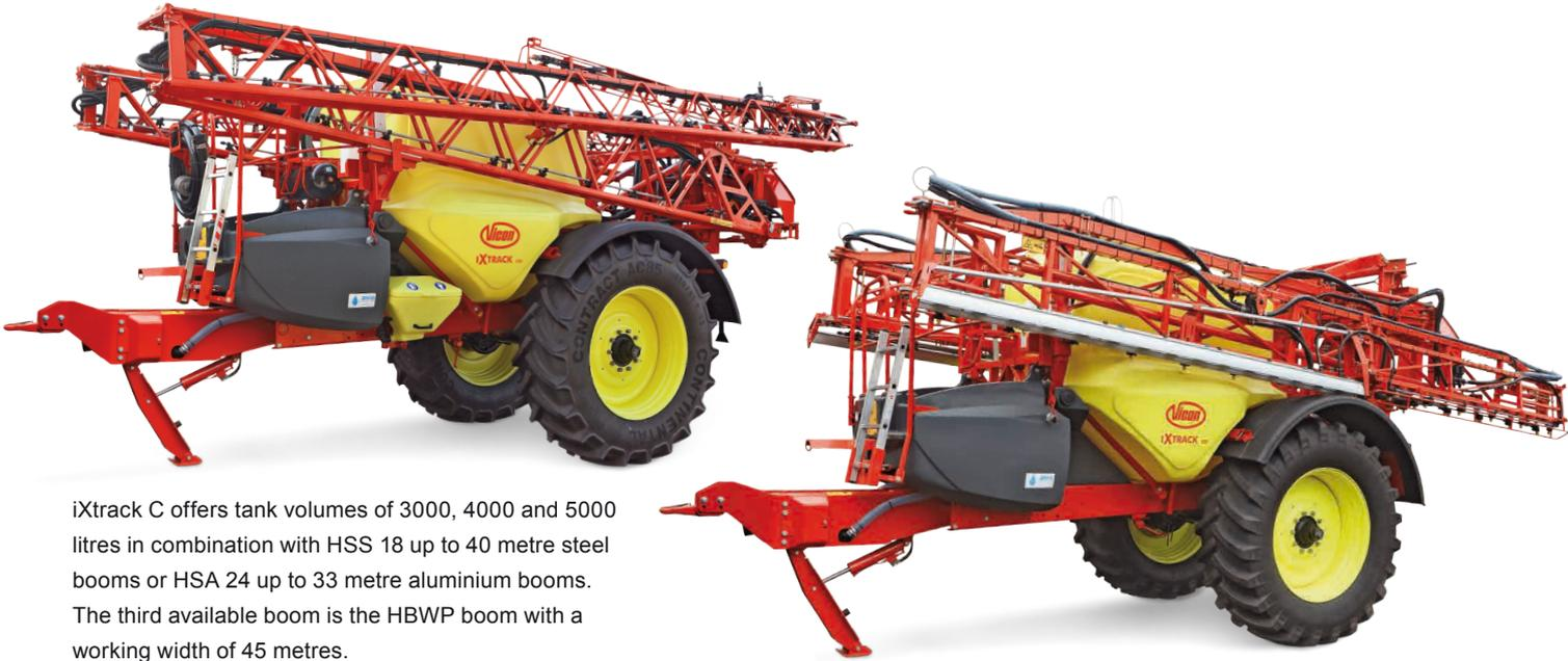
iXtrack C offers tank volumes of 3000, 4000 and 5000 litres in combination with HSS 18 up to 40 metre steel booms or HSA 24 up to 33 metre aluminium booms. The third available boom is the HBWP boom with a working width of 45 metres.
