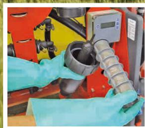
The self cleaning pressure filter prevents blocking via a continuous flow keeping the filter mesh clean. The undissolved particles are returned into the tank until they are completely dispersed.
