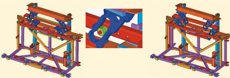
The anti yaw system provides you independent suspension left/right and is eliminating boom movements created by accelerating and braking.
