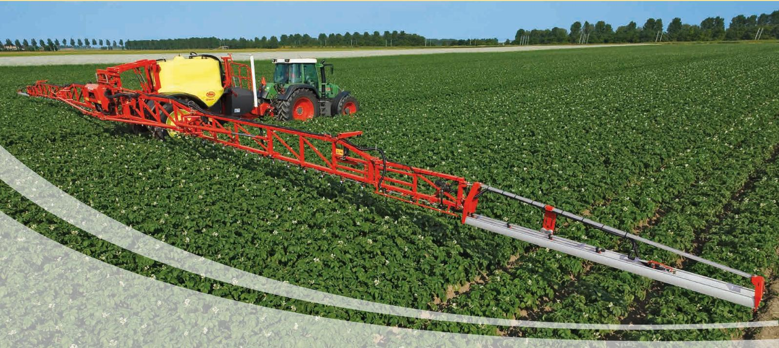
Perfect boom guiding in hilly or flatland position through a professional double trapezium balancing system. In flatland position the boom is perfectly levelled out and compensates a wrong position of the sprayer compared to the field shape. In hilly conditions the HBWP boom is following automatically the inclination of the sprayer.
