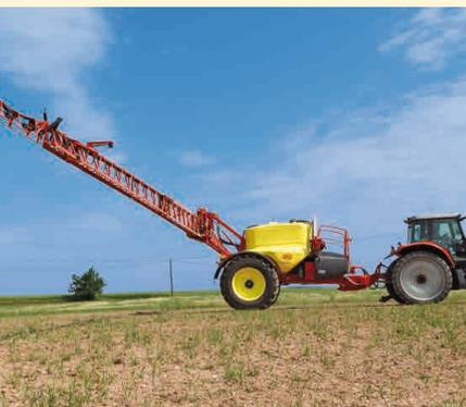
The clever tank design greatly contributes to the sprayers low centre of gravity. Short turning on the head land is possible even in hilly conditions. The parallelogram can be raised or lowered with two hydraulic cylinders with nitrogen dampers. A high clearance of 2.65m from the nozzle to the ground can be achieved!
