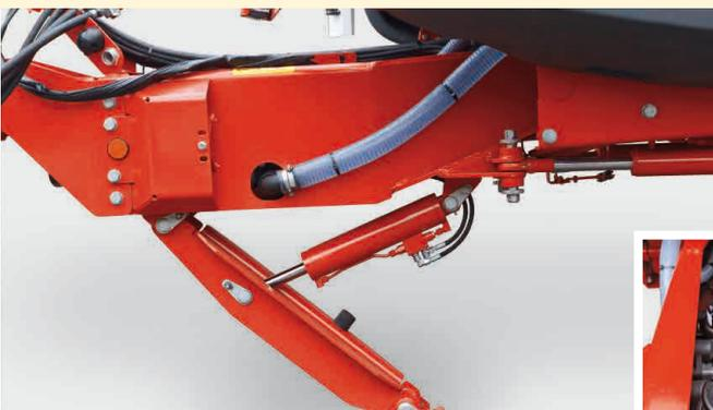
The low or top linkage drawbar with steering (unsuspended) allows short turning on the headland. Pumps are well protected and integrated in the drawbar.
