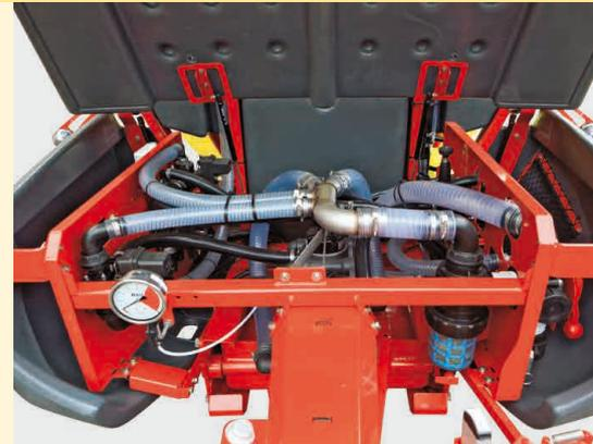
Easy access to filters, pumps, electrical and hydraulic circuits for easy maintenance.
