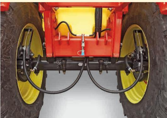
Adjustable suspended axle (iXtrack C30/C40)
