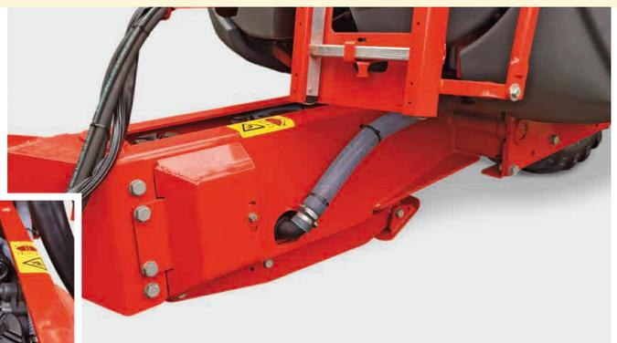
The low or top linkage drawbar with Hydroflex suspension and integrated pumps provides maximum ground clearance and well protected pumps.
