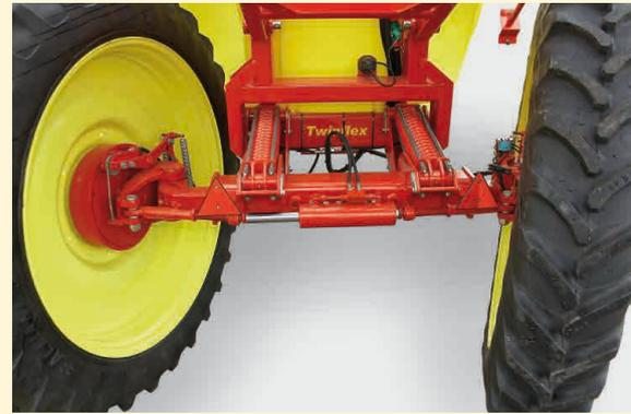
Adjustable suspended steering axle (iXtrack B)
