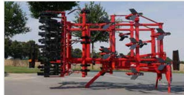
Either mounted rigid or fold – both version are very compact for a good centre of gravity and reduced lifting capacity. For safty parking extra legs are available.
