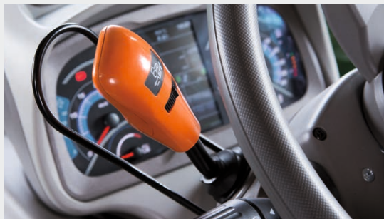
↑ Powershuttle with 5 adjustable settings for changes of direction without interruption of torque.
