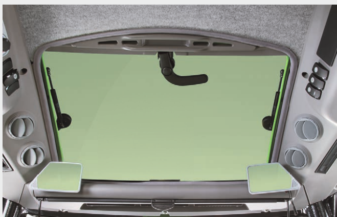
↑ A choice of four roof designs: a transparent sunroof with or without FOPS and an opaque roof with or without FOPS.
