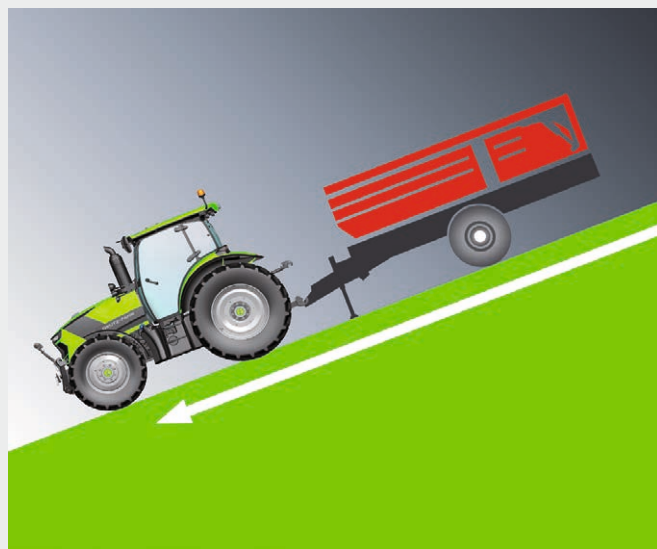
A hydraulic or pneumatic trailer brake ensures safe travelling with heavy loads.
