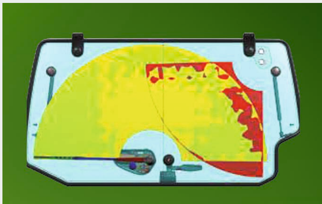
↑ Optimised wiper position on the rear screen – the best visibility in wet or dirty conditions. Now also available with defrost.
